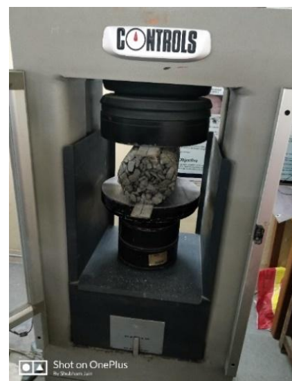
Figure 3: Testing of the sample (Just before load is applied)
